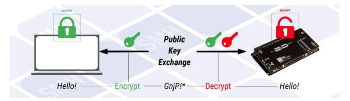
Since the pair of keys are randomly generated, each FlashRunner has its own unique keys and data encrypted for a specific FlashRunner can only be decrypted by that FlashRunner. Moreover, each FlashRunner model can only have a single pair of keys and the user can choose to regenerate the keys
