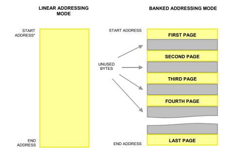
$<sup>^{\</sup>star}$  This address should correspond to the address that contains the first Flash or EEPROM data of your code. Use the Offset parameter in the FRB conversion, to set it.
