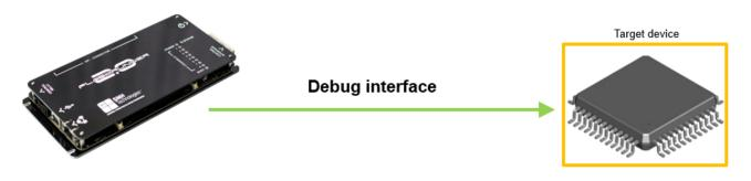
• Indirect Flashing via Application in RAM: Alternatively, the programming system may load an application into the target device's RAM. This application, once executed, will execute the flashing process by communicating with the programming system through the debug interface. RAM serves as temporary storage for the executable code, allowing the programming system to perform necessary actions, such as transferring firmware to the device's non-volatile memories.
