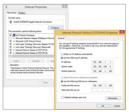
FlashRunner 2.0 Workbench is configured by default to connect to 192.168.1.100 FlashRunner 2.0 IP address. If need to change FlashRunner 2.0 IP address, you can easily update also FlashRunner 2.0 Workbench on connection settings.
