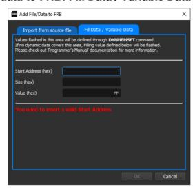
On the "Add " window there is a second tab called "Fill Data / Variable Data", the user can add a new block to FRB which contains the same value for each byte.
