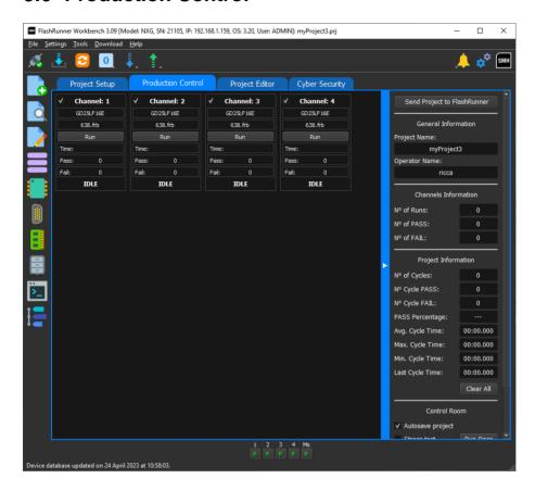
After opening a project, into the Production Control tab will be loaded a widget for each channel defined inside the project. Each widget contains the following labels:
