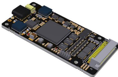
Figure 4: FlashRunner HS eMMC1/OSPI1 Active Module with right-angle device connector
