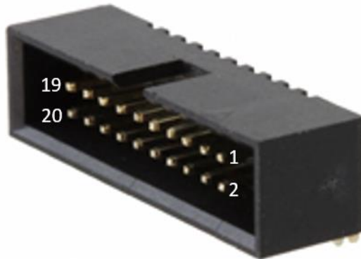
Figure 12: Control Interface connector - Right Angle, 20-position, 2-row, 1.27mm pitch – pin numbering
