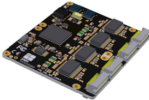
Figure 9: FlashRunner HS CAN4 Active Module with right-angle device connectors
