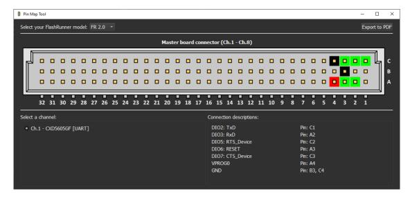
This device can support RTS and CTS flow control **only if enabled with the corresponding command**, with the configuration being the following:
